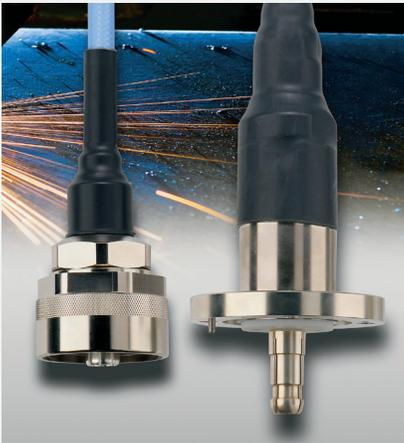
Comparison of MEIA-1625 to a comparable EIA 1-5/8 connector. MEIA™ is more than 30% smaller and 40% lighter, with a more efficient threaded coupling interface. MEIA™ line sizes are the same as EIA line sizes and can handle equivalent power.
