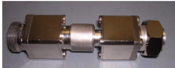
Image 2 - Mated Test Assembly for QDS(m) to QC(m)
