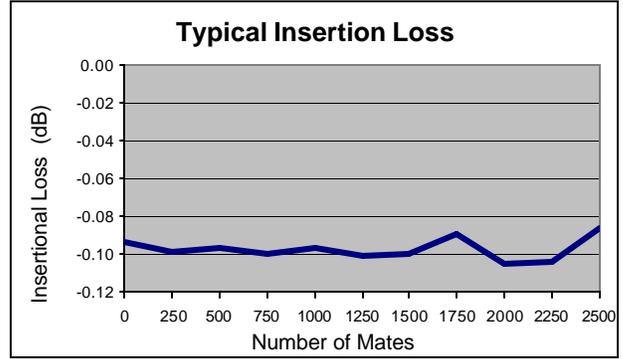
Figure 24 – Typical Insertion Loss for the QC Adapter
