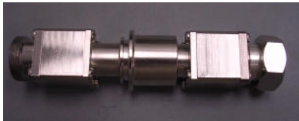
Image 6 - Mated Test Assembly for QRM(m) to QC(m)
