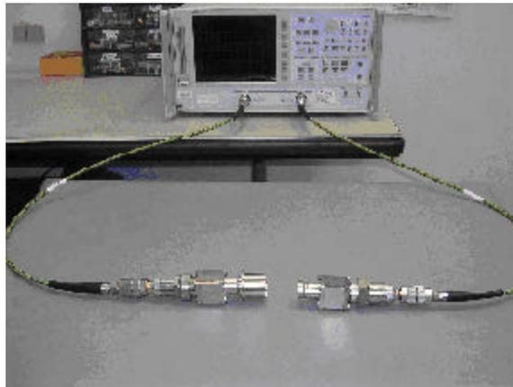
Image 12 – Vector Analyzer (HP 8753E), Test Cables, and Adapters
