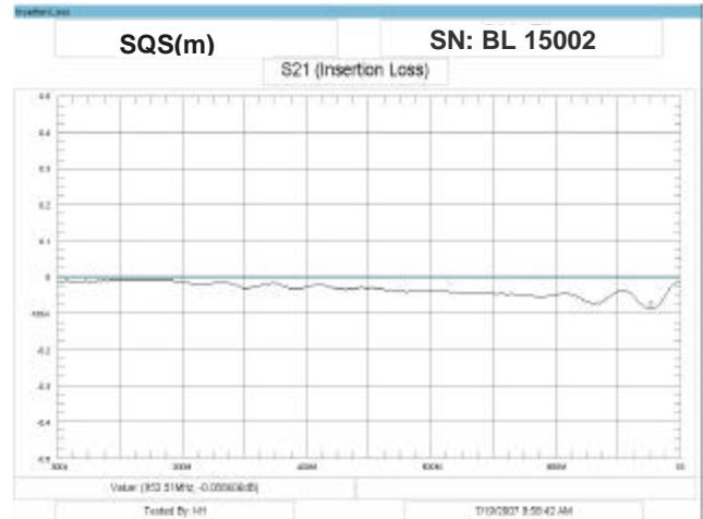
Figure 12 - Typical Insertion Loss for New SQS(m) to QC(m)
