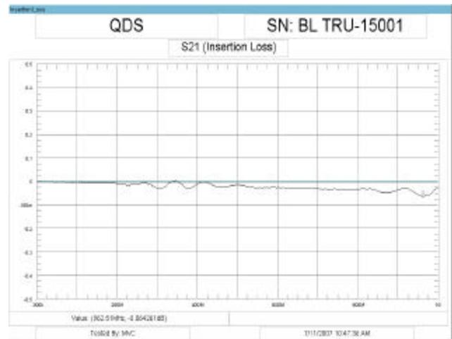
Figure 8 - Typical Insertion Loss for New QDS(m) to QC(m)
