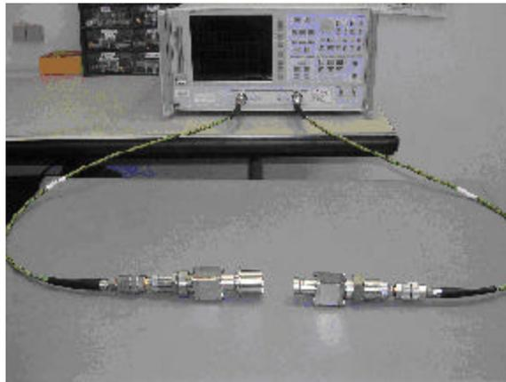
Image 11 – Vector Analyzer (HP 8753E), Test Cables, and Adapters
