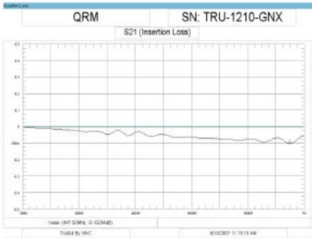
Figure 15 - Typical Insertion Loss for Original QRM(m) to QC(m)
