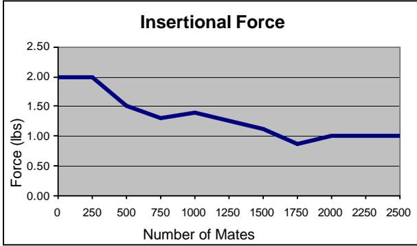
Figure 21 – Insertion Force for the QC Adapter
