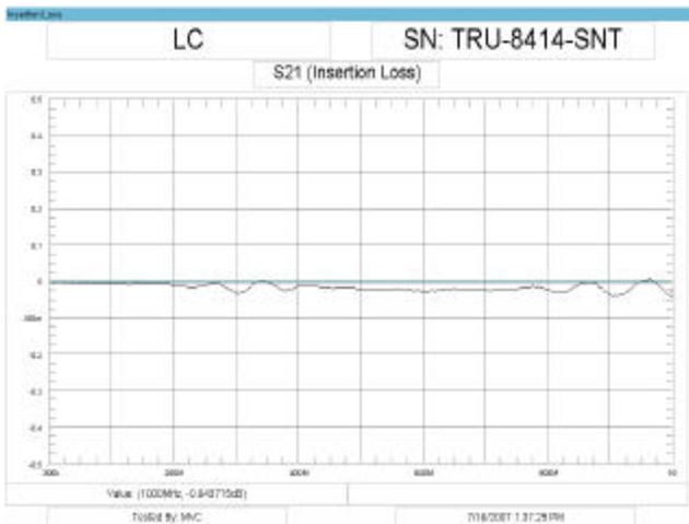
Figure 3 - Typical Insertion Loss for Original LC(f) to QC(m)
