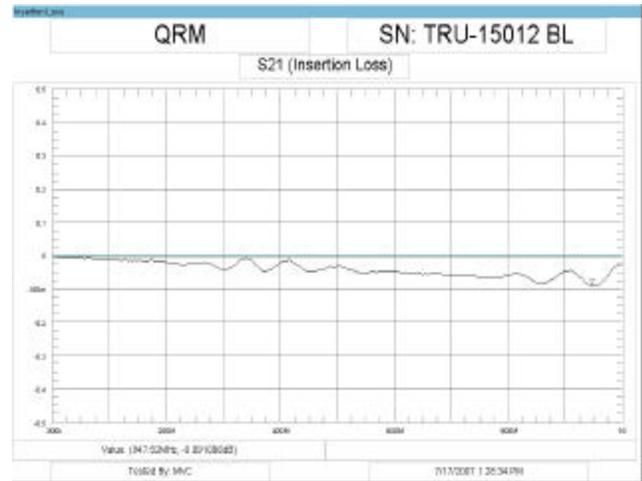
Figure 16 - Typical Insertion Loss for New QRM(m) to QC(m)
