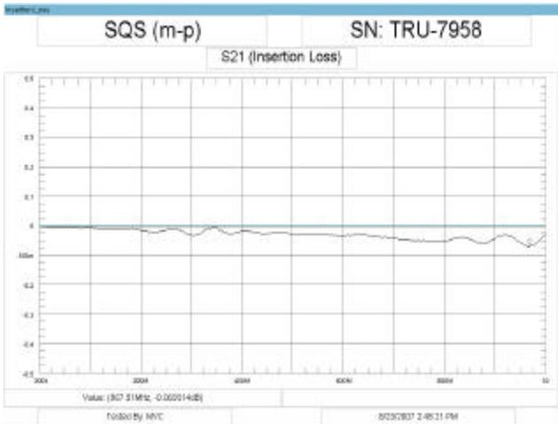
Figure 19 – Typical Insertion Loss for Original SQS(m-p) to QC(m)
