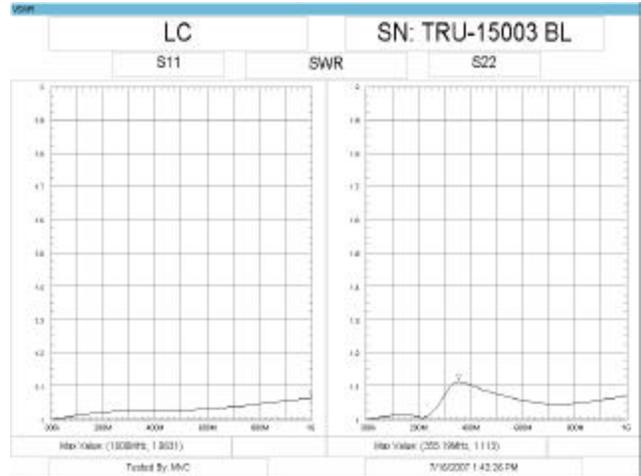
Figure 2 - Typical VSWR for New LC(f) to QC(m)
