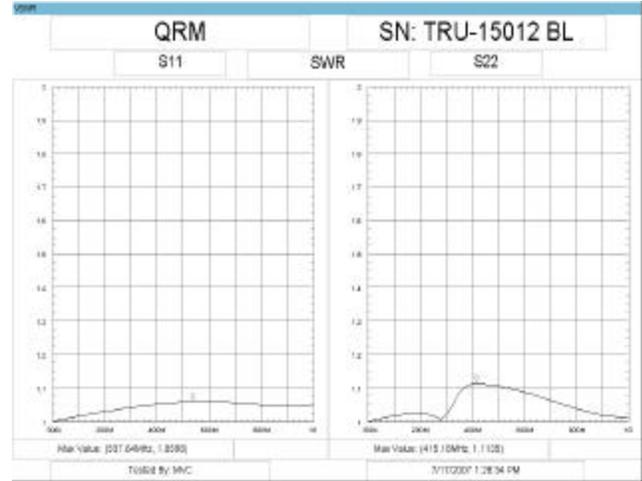
Figure 14 - Typical VSWR for New QRM(m) to QC(m)
