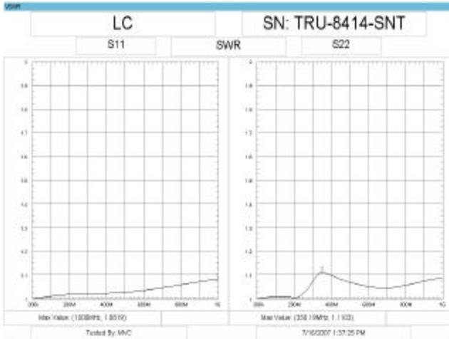
Figure 1 - Typical VSWR for Original LC(f) to QC(m)
