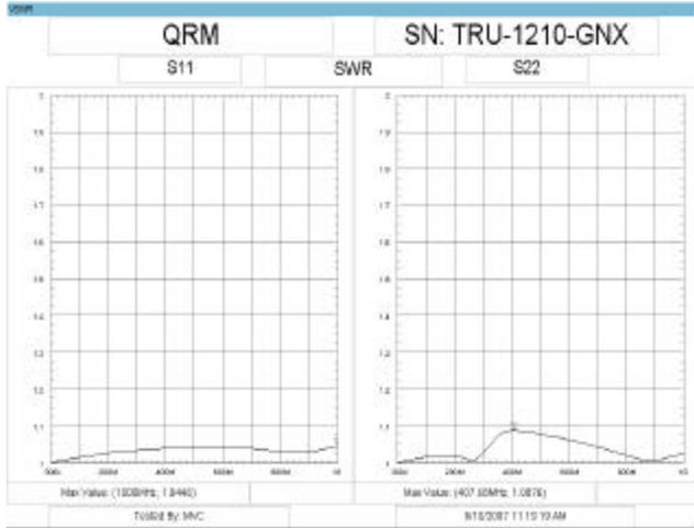
Figure 13 - Typical VSWR for Original QRM(m) to QC(m)
