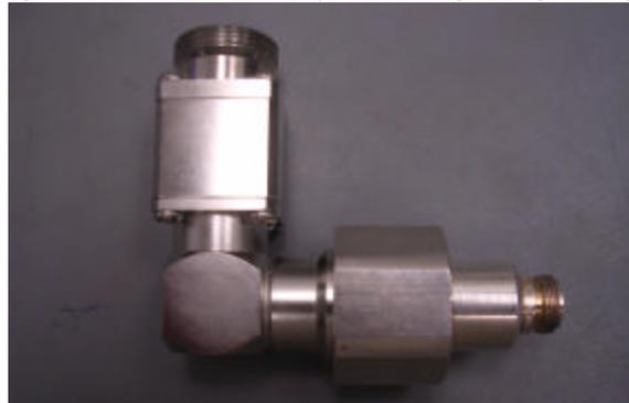
Image 10 - Mated Test Assembly for LC Right Angle Adapter
