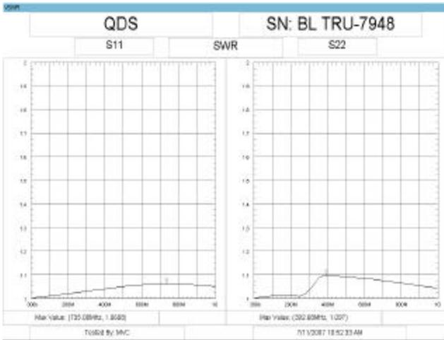
Figure 5 - Typical VSWR for Original QDS(m) to QC(m)
