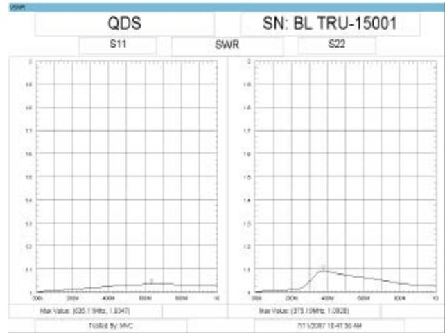
Figure 6 - Typical VSWR for New QDS(m) to QC(m)
