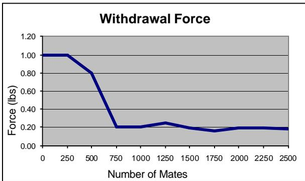
Figure 22 – Withdrawal Force for the QC Adapter
