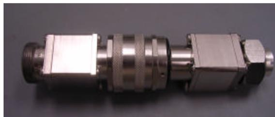
Image 8 - Mated Test Assembly for SQS(m-p) to QC(m)
