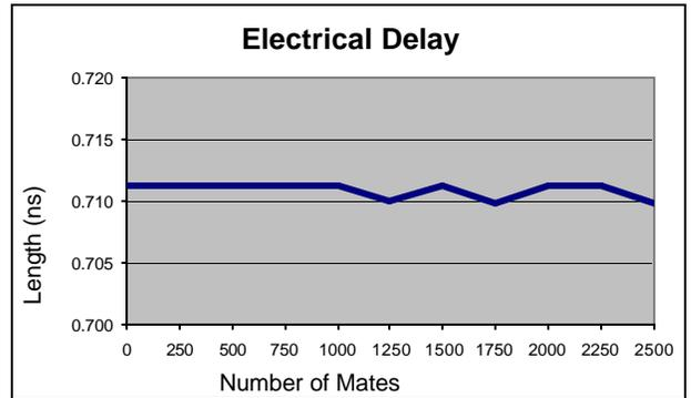
Figure 25 – Electrical Delay for the QC Adapter
