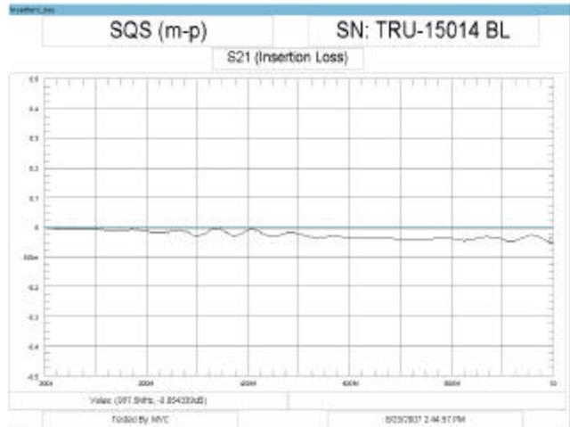
Figure 20 – Typical Insertion Loss for New SQS(m-p) to QC(m)
