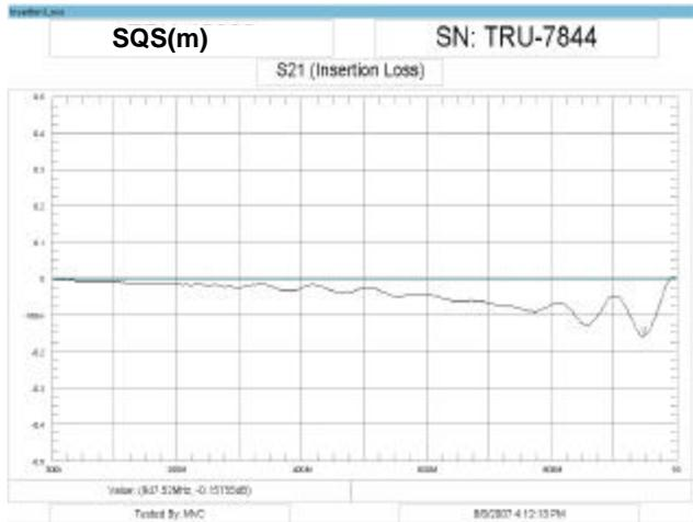
Figure 11 - Typical Insertion Loss for Original SQS(m) to QC(m)
